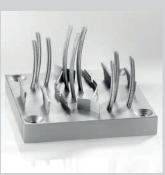
Michelin seeks to expand the Group's knowhow by constantly taking advantage of advanced innovative technologies, including – since 2006 – metal additive manufacturing. Michelin has acquired unique expertise in the design and production of the complex components used for the moulds that make the MICHELIN Road 5's siped tread pattern.
